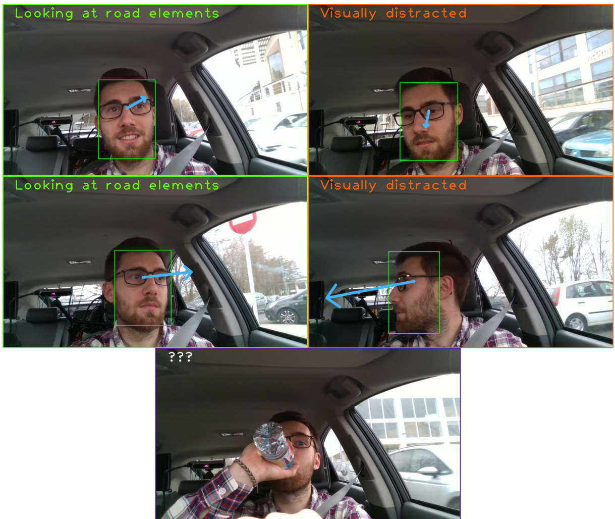
Figure 5.5: The driver monitoring system captions frames from a video by using the Gaussian Naive Bayes visual attention classifier.
